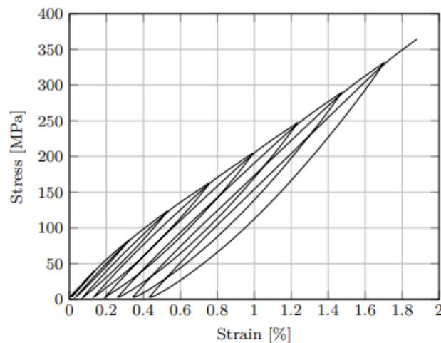
*Figure 3: Typical stress Strain Curves and Relaxation of Viscoelastic Flax Epoxy [8]*
