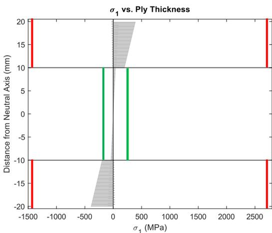
Figure 12: Stress parallel to fibres 1-direction
