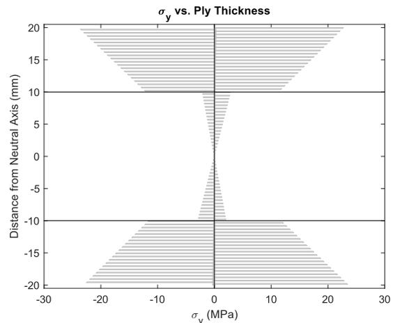
Figure 10: Stress in the y-direction perpendicular to fibres.
