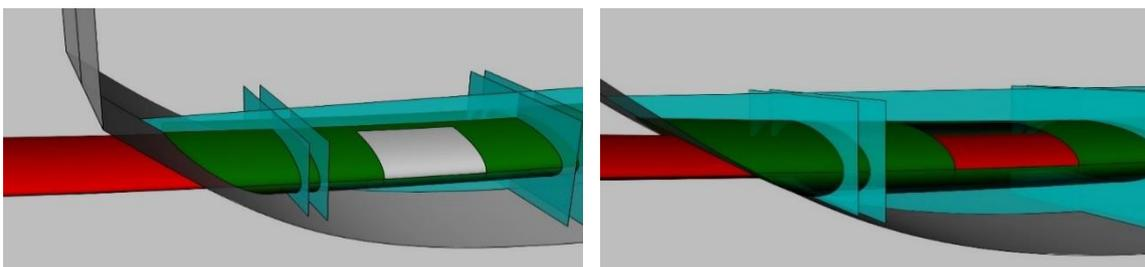
Figure 19: Starboard maintenance hatch (in grey) located on foil casing (green). Closed (left) and open (right)
