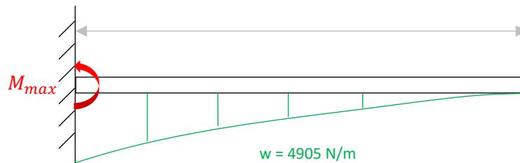
Figure 6: Bending Moment on Foil.
