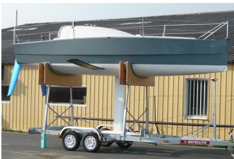
Figure 3: DSS Equipped Mini 6.50 [20].
