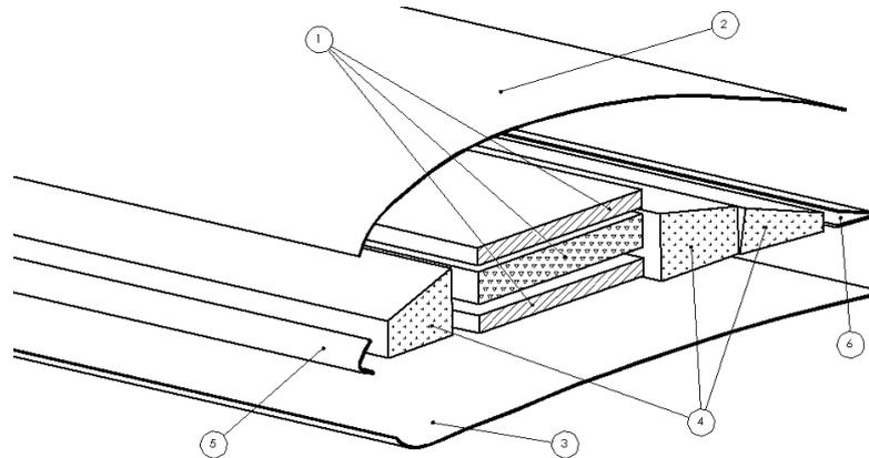
Figure 14: Exploded view of foil components
