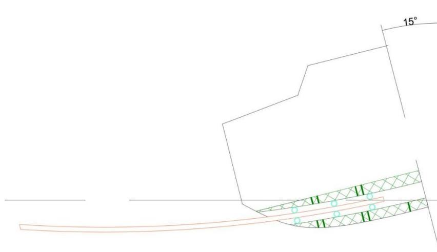
Figure 18: Deployed DSS system and its deploying system at 15° heel angle. Rubber wheels are in cyan.
