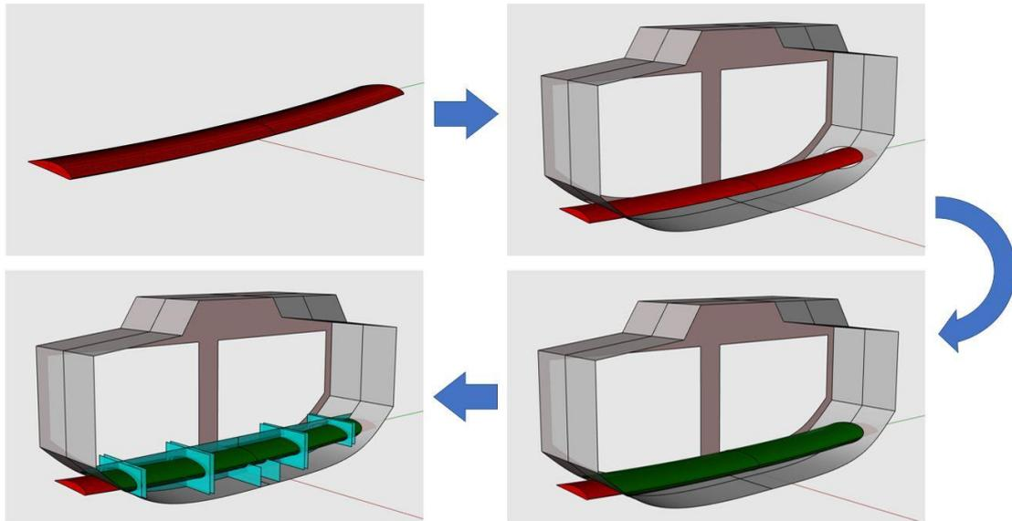
Figure 17: Flow chart diagram of the DSS supporting structure. Looking from forward to aft, the rear bulkhead is the mast bulkhead.
