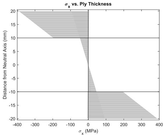
Figure 9: Stress in the x-direction (along foil span)
