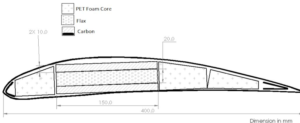
Figure 13: Cross sectional view of the foil's internal architecture
