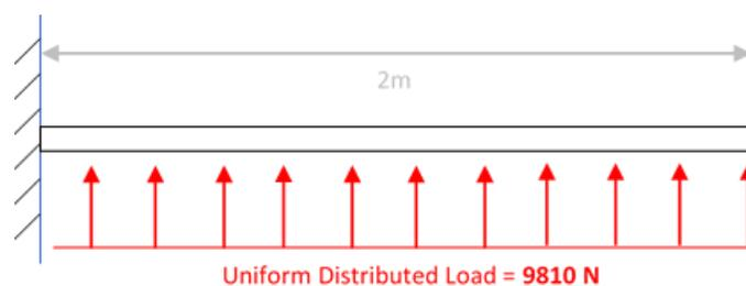
Figure 5: Uniform Distributed Load on Foil
