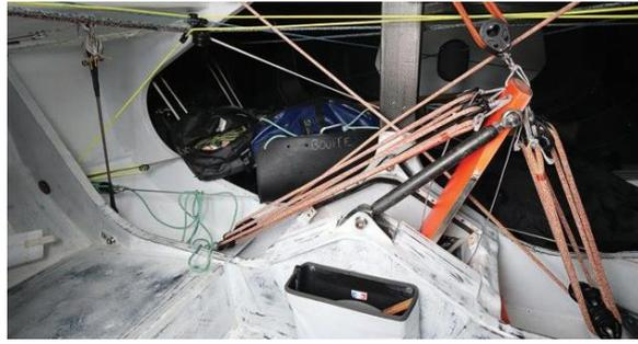
Figure 15 Interior of a Proto Mini 6.50, showing canting keel pendulum mechanism [8]
