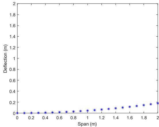
Figure 7: Foil span deflection under load.
