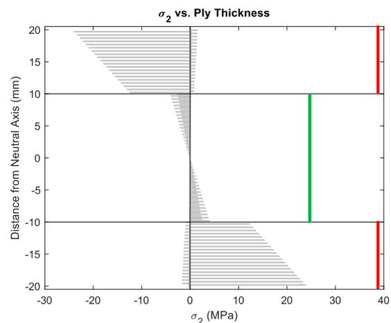
Figure 11: Stress perpendicular to fibres 2-direction
